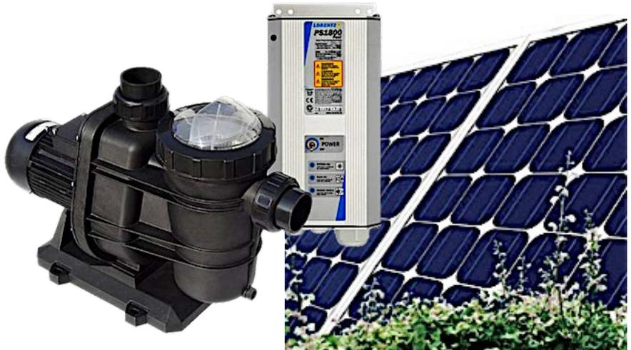
The LORENTZ pump uses a DC brushless motor for high efficiency and reliability, it is connected to a solar generator via a controller. The controller monitors the system, controls the pump speed and optimizes the amount of water pumped based on the power available.
